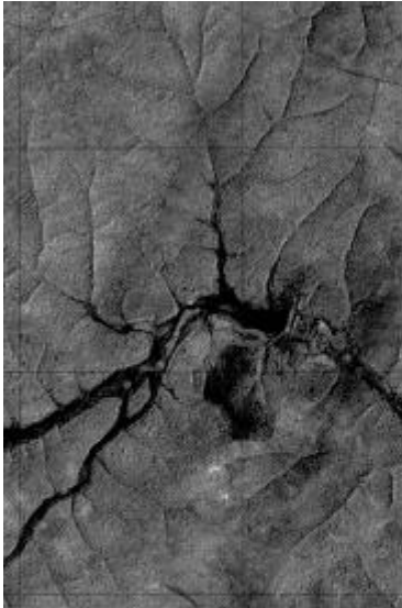
SAR-ortho-image of an area of São Francisco, Brasil produced from X-band radar data acquired by our AeS-1 instrument; the geometric resolution is 0.5 m.
