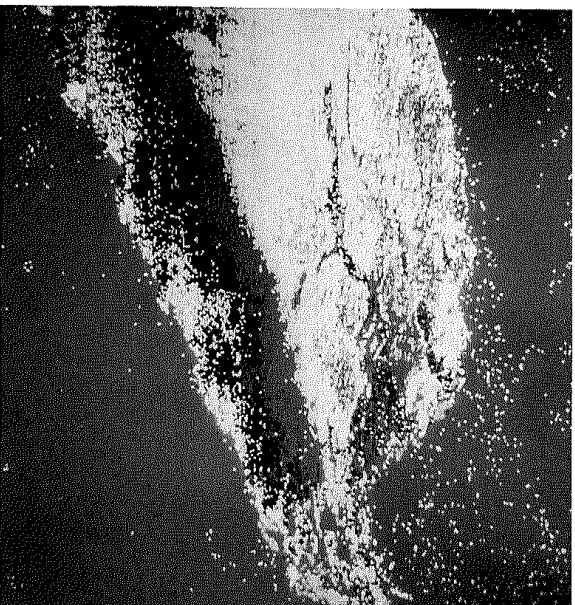
Figure 7 : The classified image for Band 4 and 5 combinations with the Euclidean Distance Classification algorithm.
