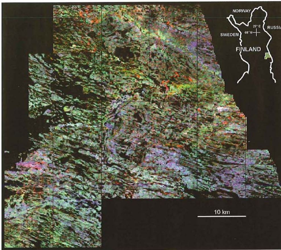
Fig. 2. Location of Kuusamo area and additive colour composite image of the airborne gamma-ray data covering the study area (eU=red, eTh=green, K=blue). (After Arkimaa 1997).
