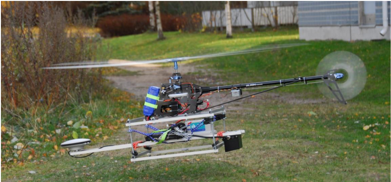
FGI Sensei mobile laser scanning system mounted on a mini-UAV
